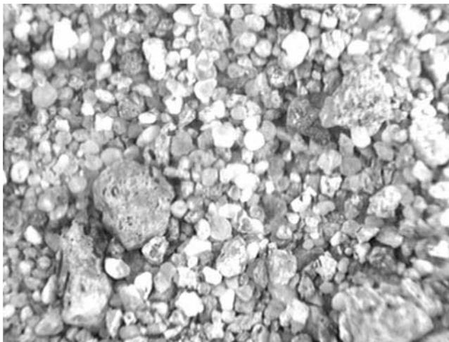
**Figure 1.** Monochrome version of FIDO Color Microscopic Imager [Haldemann *et al.*, 2002] data from May 2001 field test, showing natural soil illuminated by skylight (target in shadow). View is about 13 mm across, 20 microns/pixel, taken at  $f/10$ .
