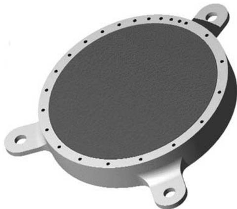
**Figure 20.** Isometric drawing of CCT. Diameter of gray disk is 45 mm; diameter of black dots around edge of target is 1 mm.
