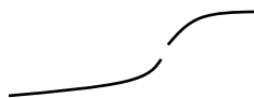
Figure 1. shows that lines can have multiple parts. This multipart line is really one feature. For an example vertex listing, see figure 4.
